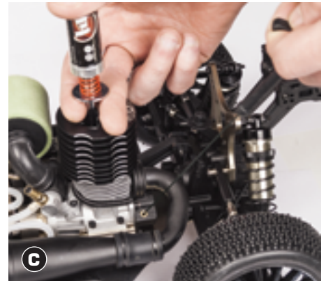
B Clamp the glowstarter over the glow plug and pull the pullstarter with short quick pulse
