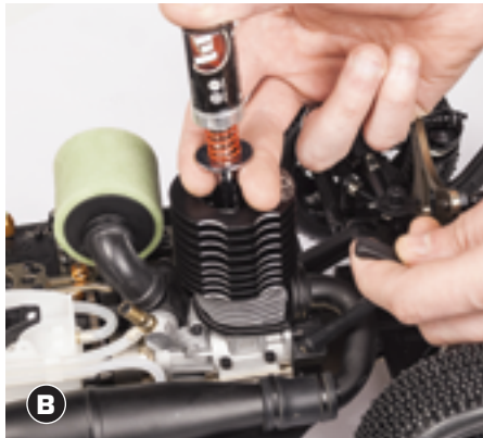
B Clamp the glowstarter over the glow plug and pull the pullstarter with short quick pulse
