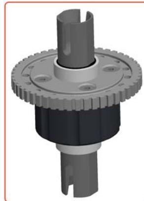
**Tighten the 4 differential screw in the cross order**
