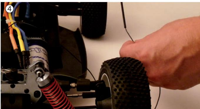
④ Slide the antenna wire into the antenna pipe carefully
